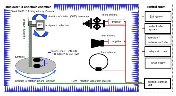
Measurement distance: tri-log antenna and horn antenna 3 meter; loop antenna 3 meter BAT-EMC software version: 3.16.0.49
