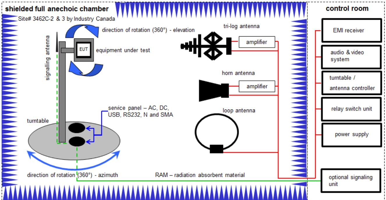
Measurement distance: tri-log antenna and horn antenna 3 meter; loop antenna 3 meter
